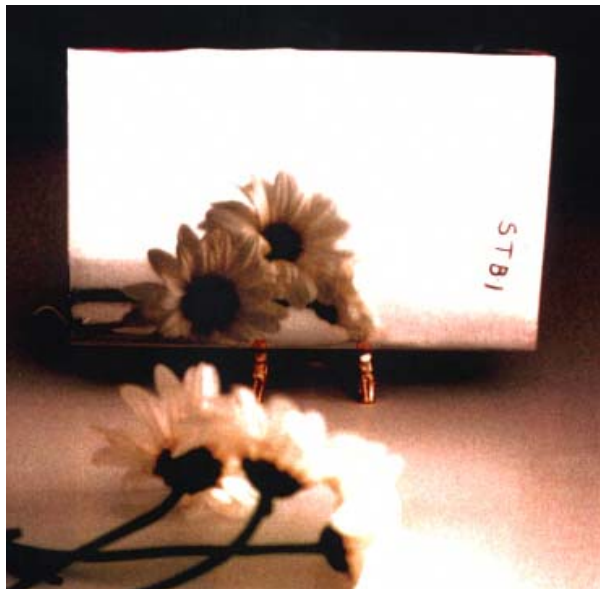
This piece of corrosion-resistant stainless steel still has a mirror-like finish after 60 years' exposure to the corrosive salt-waves and blasting winds of the Atlantic Ocean. The stainless steel for waste packages is even more corrosion resistant.
