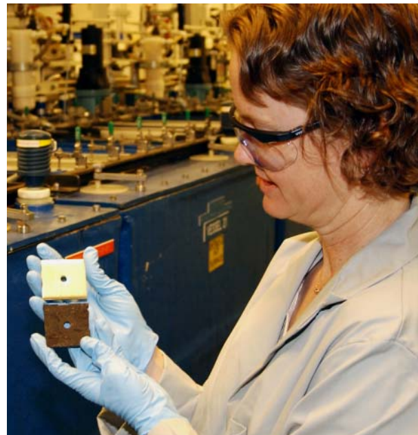
This picture shows samples of Alloy 22 and a high-quality steel, after exposure to an accelerated aging corrosion experiment. Alloy 22 is expected to lose its integrity very slowly in the repository environment.
